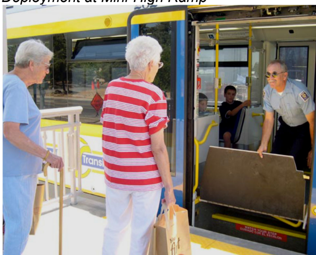
Figure 29: Bridge Plate Deployment at Mini-High Ramp
