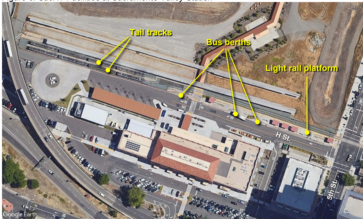
Figure 6: SacRT Facilities at Sacramento Valley Station
